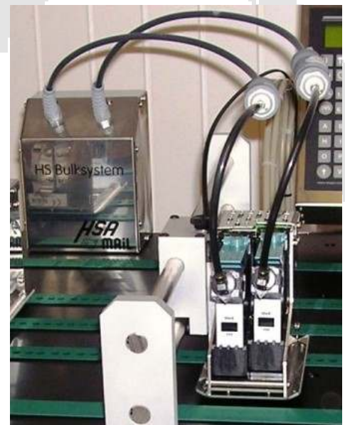
Automatic Bulk Supply System
