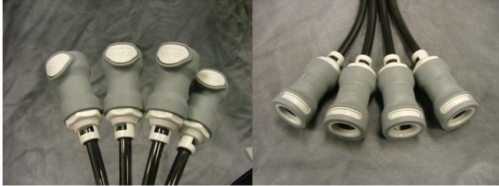
To connect ink tubes first separate them from each other at the ends. Initially you should separate about 4" (10cm) to allow for connection to fittings. Push tubes firmly but carefully over ink ports on the reservoir using caution not to break fittings. Next, install the quick connects to the other end of the tubing using the same method. Emery cloth can be used to grip the tubing better.
